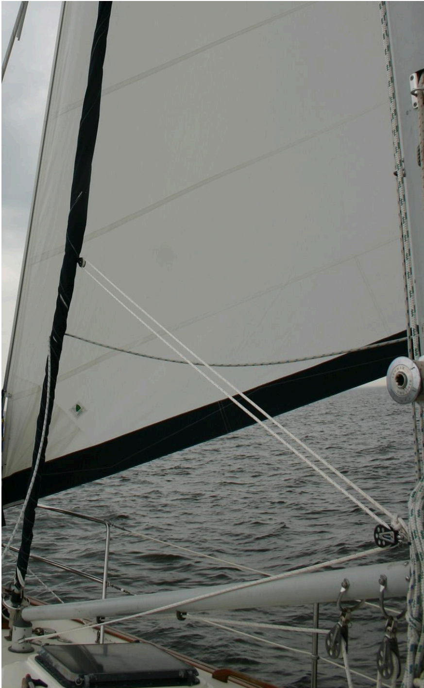
The new furling system. The outhaul runs along the boom forward then turns at the base then passes through a series of bulls eyes to the cockpit.
