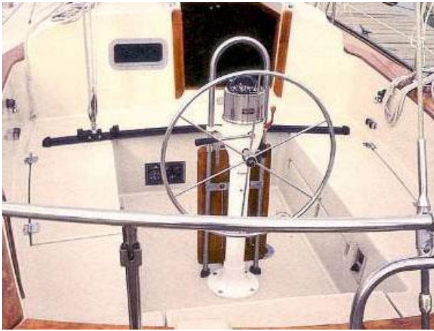
The original traveler on Sea Dragon was located in the cockpit and mounted to the boom about 4.5 feet from the end of the boom. (sister ship)
