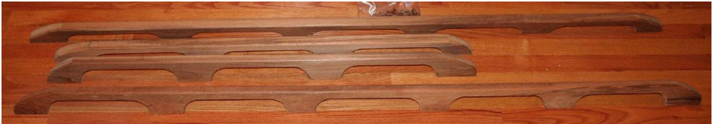
Above you can see the new hand rails.. Note the rails are NOT flat on the bottom but cut at an angle to match the slope of the coach roof so that they sit vertically.
