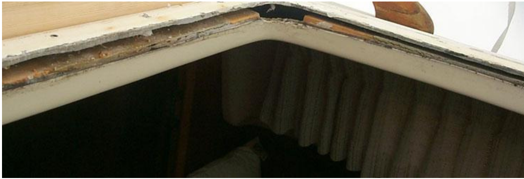
Forward Hatch (Notice the space between the liner & deck)
