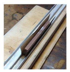
Before assembling the ports, I cleaned the channel really well water then, using a scrap piece of wood and 220 grit sand pap the channel to remove any corrosion and rough the area to all silicone to seal better.
