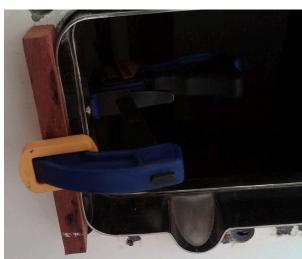
Completely compressing the butyl caulk took about 30 minutes per port. I began by tightening the screws until there was resistance. I let them port sit for 5-10 minutes while prepped the next port for installation. I would then return to the port and tighten each screw approximately one-half of a turn in a criss -cross pattern working my way from the outside edge working my way to the center.
