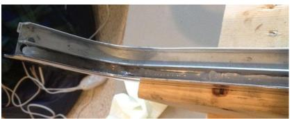
Using my simple to build jig to hold the frame in place, I applied liberal amounts of silicone to the channel.
