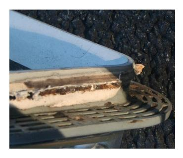
Once the ports were removed I was surprised to see how large the gap is between the coach roof and the liner. It was important to come up with a way to fill the gap. The picture on the right shows the gap on the port side of the boat. On Sea Dragon the gap is larger on the starboard side than on the port side.
