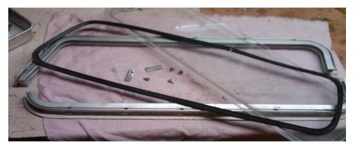
In this picture you can see the two channels. Once disassembled it is easy to see that water has been coming in around the window for some time. The corrosion can be seen clearly in the window channel (top).
