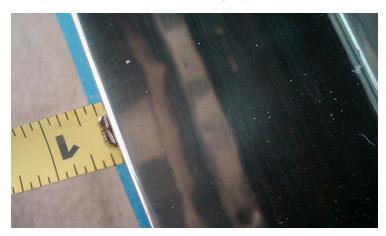
Now with opening cut and filled, I cleaned the liner, coach roof, SS steal trim ring, and the portsusing acetone. My plan was to clean anything the butyl would touch or the sealant.
